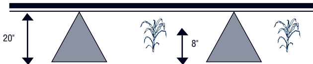
Diagram 1: Spray pattern of an even spray nozzle for inter-row applications.
